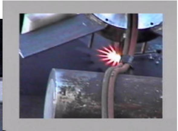
Design of WallWalker's tool carrier allows it to be readily adapted to well established, conventional processes which have been demonstrated to effectively and economically produce the desired result. The cutting torch used here is a propane fueled system commonly found in shipyards and fabricating plants; oxyacetylene or gasoline torches could be accommodated with similar ease.
