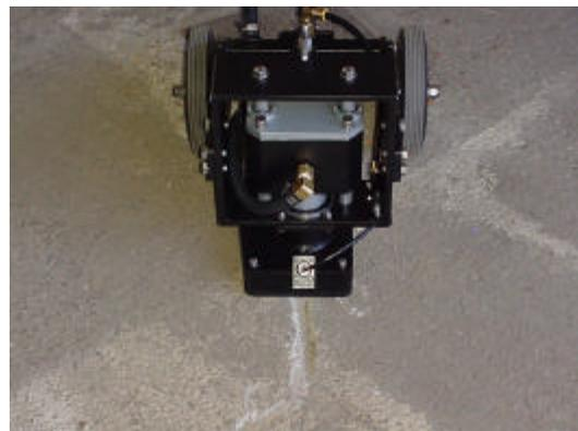
\*6-inch wheels allow for control with fingertip ease in forward, backward and side-to-side motion.
