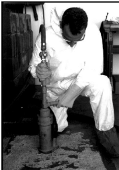
The **SQUIRREL-I** can handle hard epoxies or mastic coatings, combining the power of a sledgehammer with the advanced cleanliness provided by a vacuum attachment designed for radiological decontamination.
