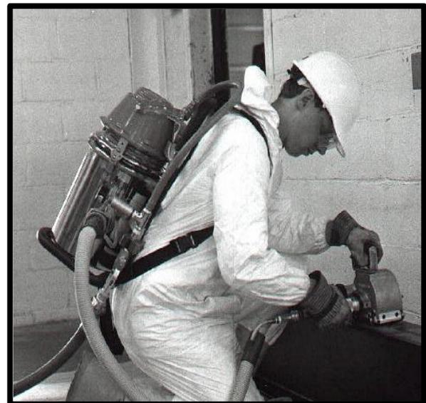
The **COMPACT-VAC** collects all dust and debris as the **ROTO-PEEN SCALER** prepares steel, concrete, brick and wood surfaces at a nominal rate of 45 sq. ft./hr.
