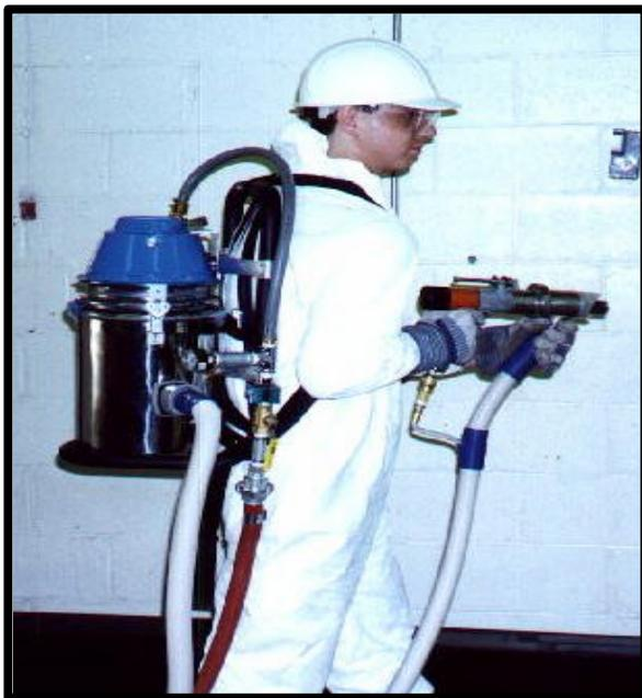
The **COMPACT-VAC** supports Pentek's shrouded power tools, including the **CORNER-CUTTER** needle gun, which comes equipped with multi-geometric shrouds for corners, edges and bolts.
