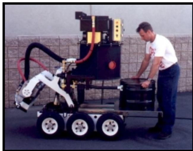
*MOOSE® integrates an on-board vacuum which is closely coupled to the concrete scabbling head. The result: a compact, efficient design with automated controls to eliminate operator exposure to hazardous materials.*
