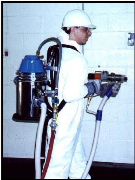
The COMPACT-VAC supports Pentek's shrouded power tools, including the CORNER-CUTTER needle gun, which comes equipped with multi-geometric shrouds for corners, edges and bolts.
